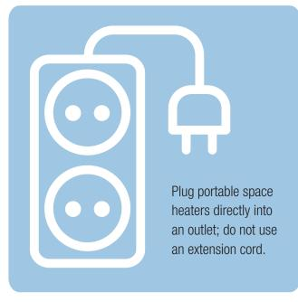
Make certain the circuit you plug a space heater into can adequately and safely handle the added demand.
